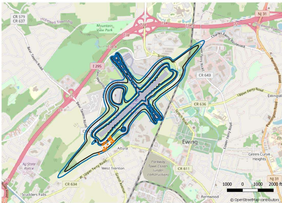
Figure 7 2027 No Action 2027 65, 70 and 75 dB DNL Contours (blue) Compared to 2019 Existing Noise Contours (black)
